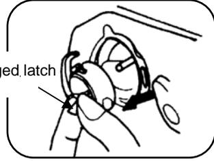
2. Open the hinged latch of the bobbin case and pull the bobbin case out of the machine.
