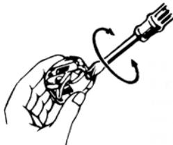
Lower thread tension can be increased by turning the screw of the bobbin case slightly to the right (clockwise). Turning it to the left (counter-clockwise) decreases tension.
