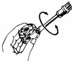
Lower thread tension can be increased by turning the screw of the bobbin case slightly to the right (clockwise). Turning it to the left (counter-clockwise) decreases tension.
