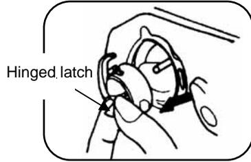
2. Open the hinged latch of the bobbin case and pull the bobbin case out of the machine.
